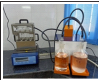
CRUDE PROTEIN DIGESTION AND DISTILLATION UNIT
